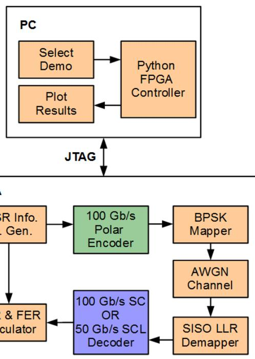
Figure 1: Demo block diagram
